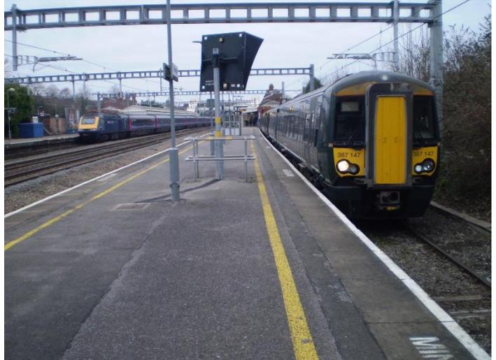
A GWR Class 387 on a Reading - Newbury service calls at Newbury Racecourse. The doors in the 4<sup>th</sup> car (nearest) do not open despite the platform being long enough.
