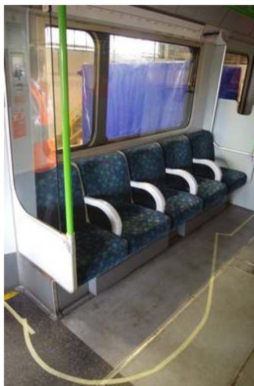
Picture on right shows the location of the toilet marked out on the floor in an unmodified interior with seating as used with London Underground.
