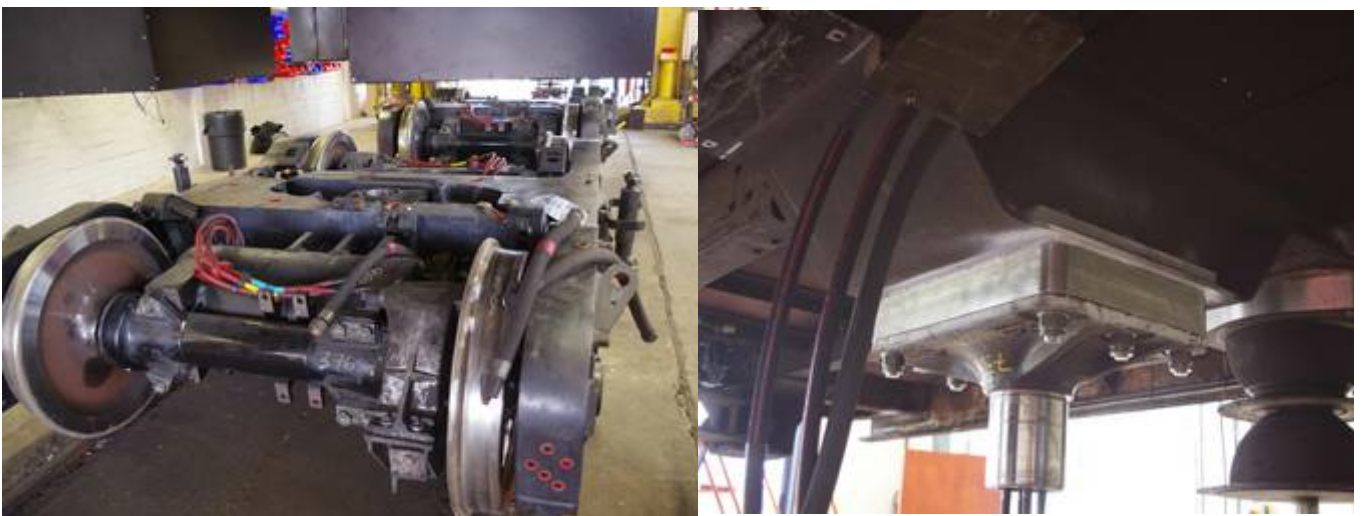
Existing bogie and pivot
