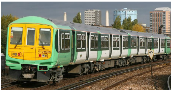
Dual-voltage Southern Class 319 on third rail power
