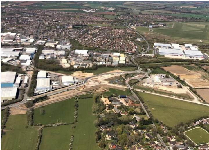
Launton Road Bicester Centre of aerial photo shows the site of a new overbridge for Charbridge Lane with temporary road diversion in place while bridge is constructed. Westwards view towards site of new road overbridge being constructed for Charbridge Lane eastern ring road.
