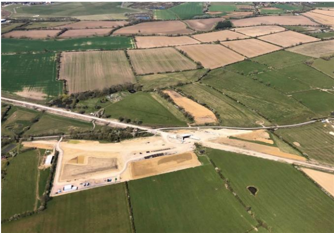
Launton The EWR route runs diagonally from left (west) to right while, in the centre, work continues on building a new overbridge for a realigned Station Road. The existing road is closed until mid 2022. New road overbridge under construction from ground level.
