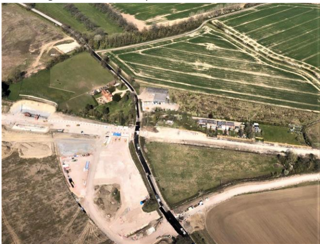
Claydon Junction Early stage of new bridge construction for Queen Catherine Road to replace existing level crossing in centre of picture. New bridge foundations are on the centre left of aerial picture. Former Claydon station site is to the right of level crossing. Ground level, looking east towards the above site from remains of the disused Claydon loop.
