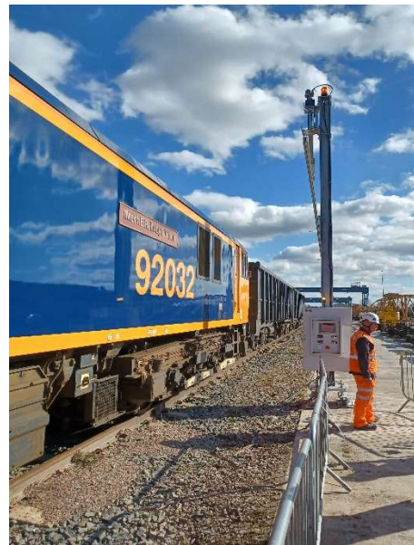
...now you don't – well, sort-of. The overhead bar is swung out of the way, to enable safe loading and unloading of the wagons.
