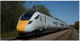
Hitachi's DfT-specified class 800 series 140mph-capable, HS1-compatible electric or electric / diesel bi-mode. Note: EMR 'Aurora' class 810 carriages (p.1) 24m not 26m. (other products may become available!)
