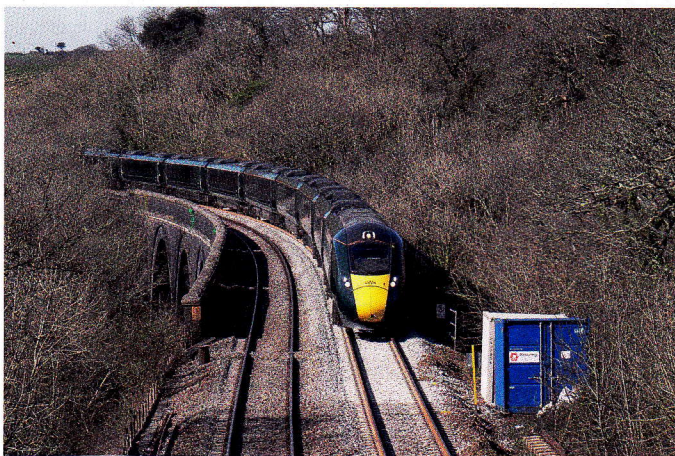
Successful blockade in Cornwall: on 7 March 2021 GWR's No 802106 working the 10.18 Penzance to Paddington passes the track renewal site at Tregarne near Probus; a temporary speed restriction (TSR) of 50mph was in place over the new track. Craig Munday
