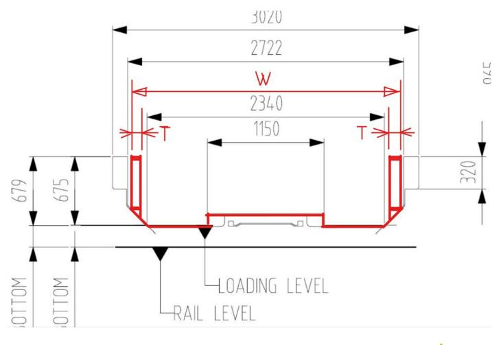
Dimensions are in millimeters: mFitting within lower part of UK Loading Gauge
