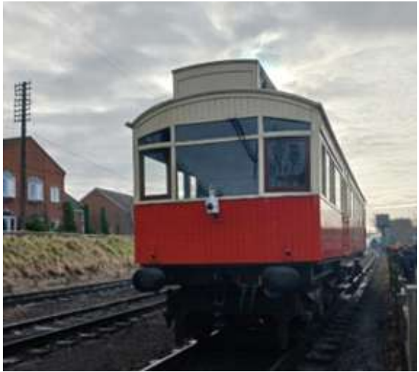
NER 'Electric Autocar' (originally petrol-electric, but now equipped with a Cummins diesel engine), lays over north of Loughborough Central prior to working the 12:15 to Rothley Brook, these vehicles were quite some way ahead of their time.
