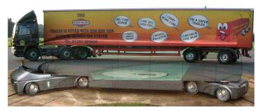
So, how does this invention help rail campaigners? Put simply, existing road-rail vehicles, which are tend to be vegetation clearance and track maintenance, are quite short. The BladeRunner bogies can be coupled to any body configuration allowing lorries and coaches to run on railway lines as long as there is a flat surface on which vehicles and join and leave the track.
