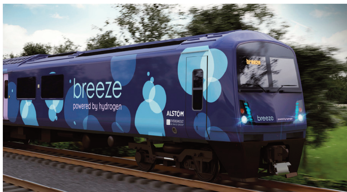
Eversholt's Breeze hydrogen train, based on a class 321 electric multiple unit
