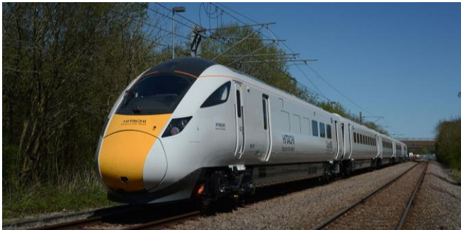
Hitachi’s DfT-specified class 800 series 140mph-capable electric or electric / diesel bi-mode.
